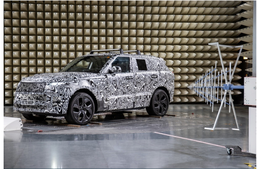
NEW ELECTROMAGNETIC COMPATIBILITY TEST FACILITY
